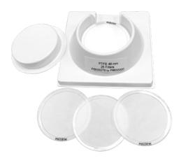
GVS Life Sciences PM 2.5 PTFE Membrane is a high-purity, thin membrane for PM 2.5 ambient air monitoring. Each membrane is sequentially numbered with a chemically resistant polypropylene support ring. The low tare mass allows for accurate gravimetric determinations. No glues or adhesives are used in making the membranes and its stable design eliminates curling, keeping the membrane flat allowing for robot use.
