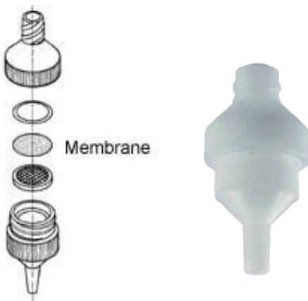
The GVS Swinney 13 mm filter holder is optimized for small volume (1-5 mL) particulate removal from fluids dispensed with a syringe. The holder is resistant to alcohols, esters, ethers, glycols, aromatic hydrocarbons, halogenated hydrocarbons, ketones, oils, photoresists and many other chemicals. Although suitable for most weak acids and bases, we recommend that you test for compatibility with acids.
