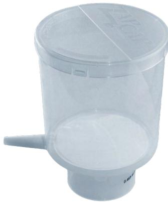
GVS Bottle-top Filters is ideal solution for the filtration of cell culture media and HPLC media solution. ZapCap is a complete 500 mL filtration unit to connect with receiver bottles. ZapCap are equipped with side tubing nozzle (bottle-top). This ready to use filter is available with prefilter too. The connection seals fit on any standard bottle 33 to 45 mm and the membrane diameter is 76 mm with an effective area of filtration of 39.2 cm<sup>2</sup>. Can be used up to 50°C.
