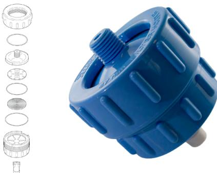
The GVS polypropylene 47 mm filter holder is designed especially for ultra cleaning and sterilizing liquids under positive pressure. In addition this holder can be used for aseptic sampling of liquids or gases at point-of-use or when samples must be collected and processed on-site. The polypropylene material allows these holders to be used over a wide temperature range with excellent chemical compatibility. Sealing is achieved by simple hand
