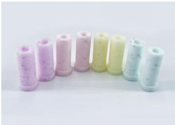
GVS cannula filters, commonly used in dissolution processes at the ends of the sampling cannula, help keep particulates from backing up into the tubes.
